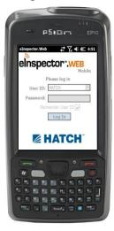
Use of PDA adds to the portability of the data collection and integrated ISO criteria make condition assessment on site simple
